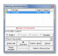
Fig. 4.1-7 Locked route because of inactive booster
